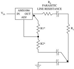
\*CONNECT R1 TO CASE CONNECT R2 TO LOAD
