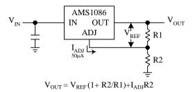
Figure 1. Basic Adjustable Regulator
