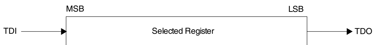
Figure 56-3. Shifting data through a register
