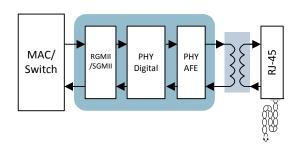
Figure 2-5. External Cable Loopback
