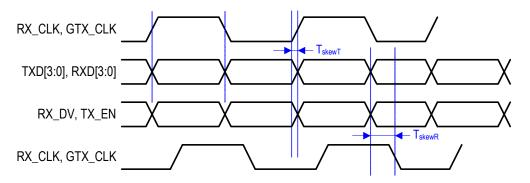
Figure 3-1. RGMII AC Timing Diagram — no Internal Delay
