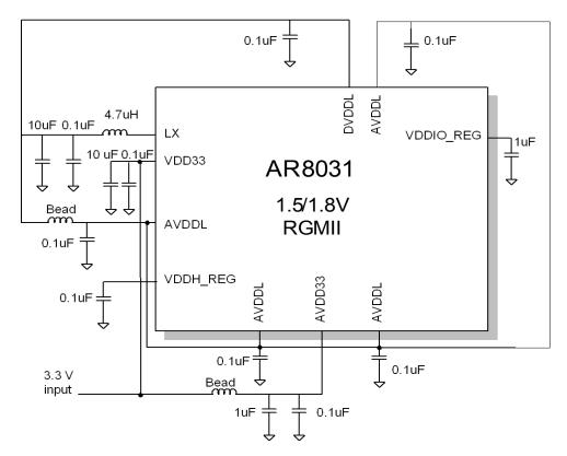
Figure 2-11. Reference Design, 1.5/1.8 V RGMII I/O
