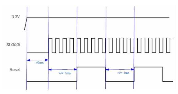
Figure 3-5. Reset Timing Diagram
