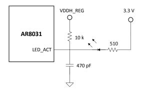
The active status of LED\_ACT and LED\_LINK1000 depends on power-on strapping mode. When the interface is strapped high, the LED interface are active low; when strapped low, active high. The active status of LED\_LINK10\_100 depends on LED\_LINK1000 power-on strapping mode and thus LED\_LINK10\_100 and LED\_LINK1000 use the same LED reference design.
