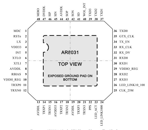
Figure 1-1. AR8031 48-pin QFN Pinout Diagram (Top View)
