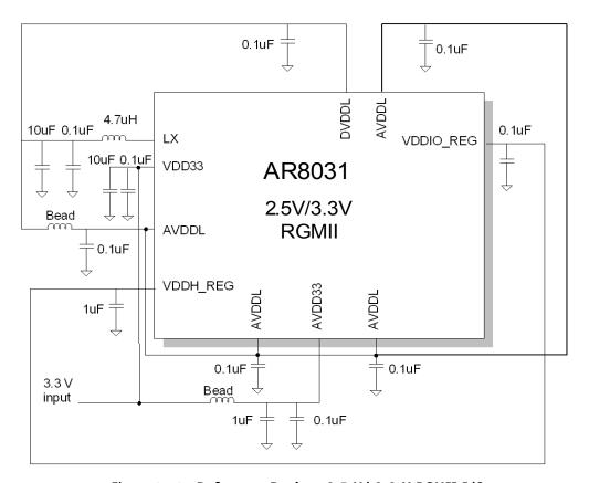
Figure 2-10. Reference Design, 2.5 V/ 3.3 V RGMII I/O
