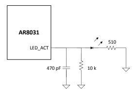
Figure 2-8. Reference Design for LED, Active High
